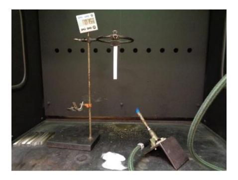
Photo No. 1 50W (20 mm) Vertical Burning Test Set Up
